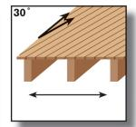
At a 30° angle, maximum joist spanning is 1/2 of the above chart.
