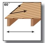
At a 60° angle, maximum joist spanning is 2" less than above chart.
