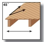
At a 45° angle, maximum joist spanning is 4" less than above chart.
